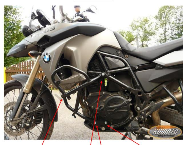
bolt M8x30mm to connect both sides
