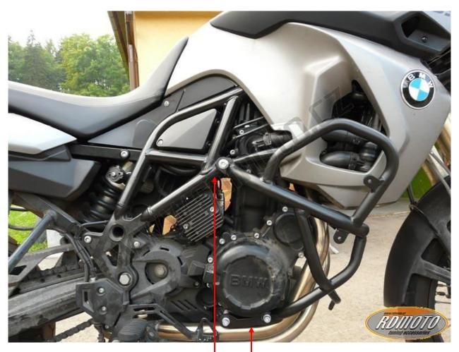
bolt M10x100mm + duralumin cylinder 32,5mm
